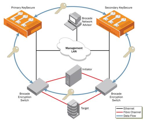
Figure 1. Components of the Brocade-SafeNet solution
