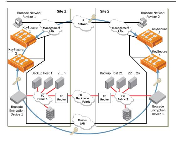
Figure 5. Data mirroring, encryption, and key management spanning two sites
