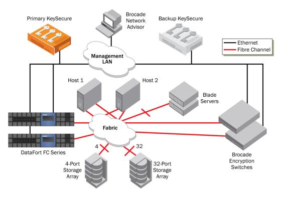
Figure 8. Upgraded deployment
