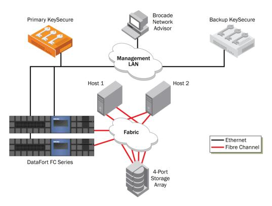
Figure 7. Initial deployment
