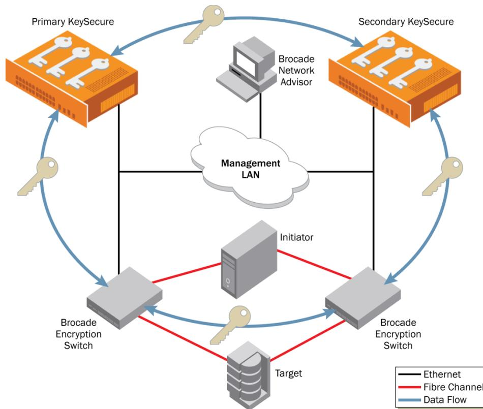
**Figure 1.** Components of the Brocade-SafeNet solution
