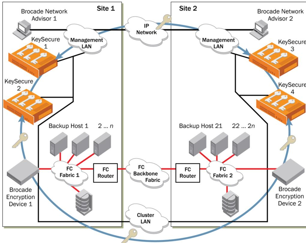
**Figure 5.** Data mirroring, encryption, and key management spanning two sites
