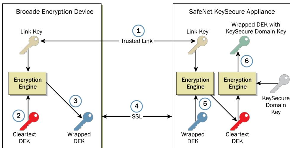
**Figure 2.** Key exchange between a Brocade encryption device and SafeNet KeySecure
